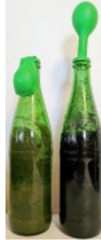
Figure 2. Aerobic, both: Sand on left, loam on right.
